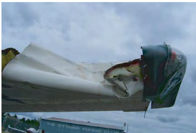
This is the second damaging bird strike this Rockwell Commander has suffered in less than 10 years. The bird was struck at 1,500 AGL and at about 130 kts. (Photo courtesy B. Mackinnon, Transport Canada)
