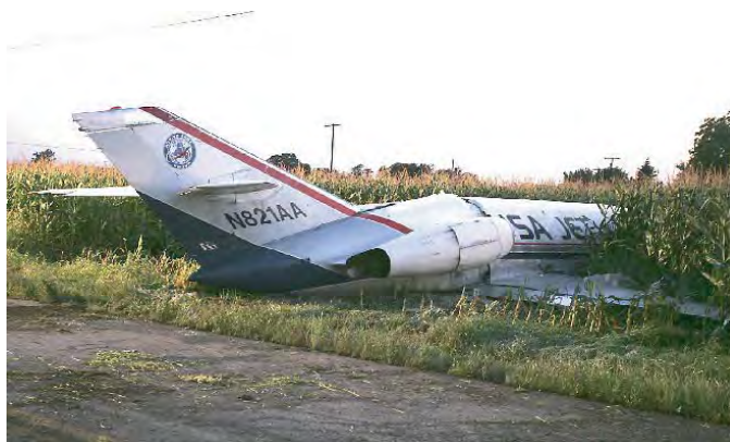
This Falcon 20 ingested at least four mourning doves into the #1 engine and five into the #2 engine during takeoff from a midwestern airport. About 20 dove carcasses were picked up on the runway at the strike site. The aircraft was damaged beyond repair. Mourning doves weigh about 4 ounces (120 grams). (Photo courtesy USDA)
