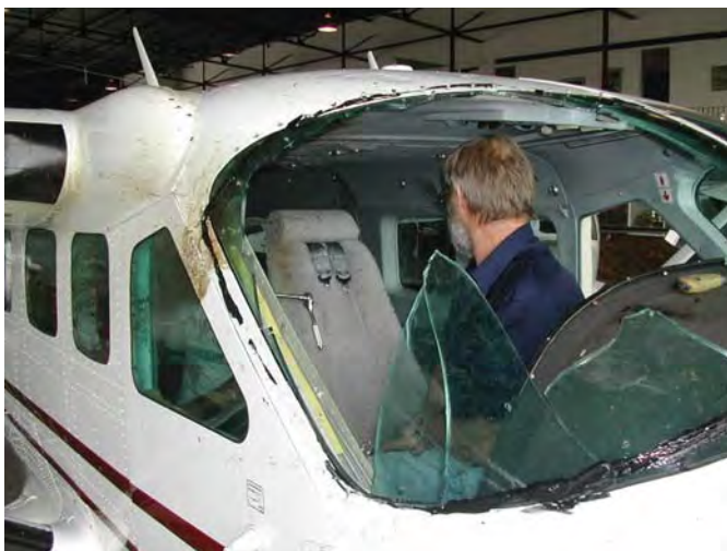
This Cessna 206 struck a single vulture on takeoff from a southern U.S. airport. The bird penetrated the windshield, severely injuring the pilot.
