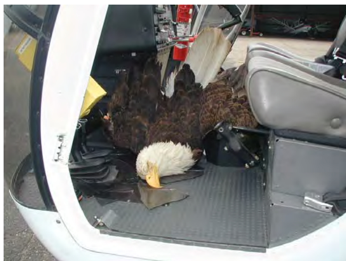
This helicopter was traveling at 80 MPH when it struck a bald eagle at 2,000 ft AGL. The eagle penetrated the windshield, striking a passenger in the chest. (Photo C. Cooper, Hummingbird Helicopters)
