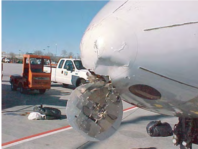
On approach to an eastern U.S. airport, this CRJ with 35 people on board sustained a goose strike to the radome, at 250 knots. There was major damage to the radome and electronic components. (Photo courtesy FAA)
