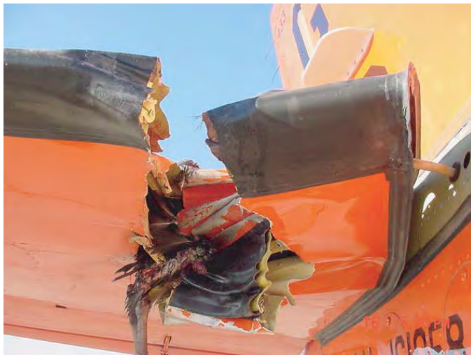
This Navy T-44 trainer struck a turkey vulture while conducting low-level training exercises near Corpus Christi, TX. The student pilot was able to land safely.
